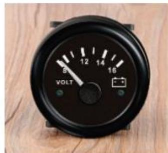
EL VOLTAJE TIENE QUE MARCAR ENTRE 13 Y 14 VOLTS
